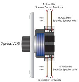
The VCRI connects with simple plug-in screw terminals. Using 16AWG (min) 2-conductor stranded speaker wire connect the amplifier speaker OUT to 'From Amp' on the VCRI. Connect 'From Speakers' on the VCRI to the left and right +/- speaker terminals.
