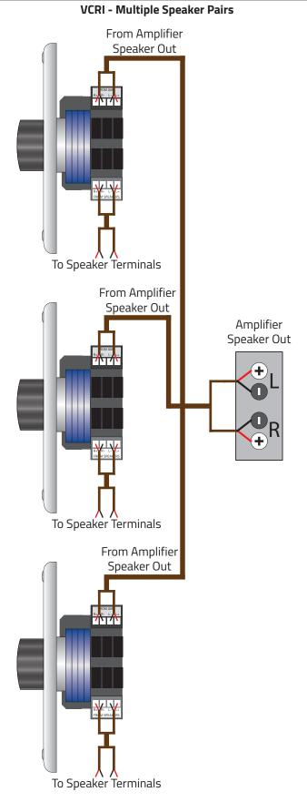
The VCRI is an automatic impedance matching volume control. Multiple VCRIs and speaker pair can be connected to an appropriately powered amplifier. There are no jumper or switch settings as long as the overall load does not exceed the amp's capability.
